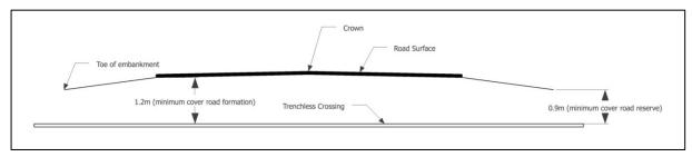
Figure 5.2.2(b) – Minimum depth below dual carriageway
