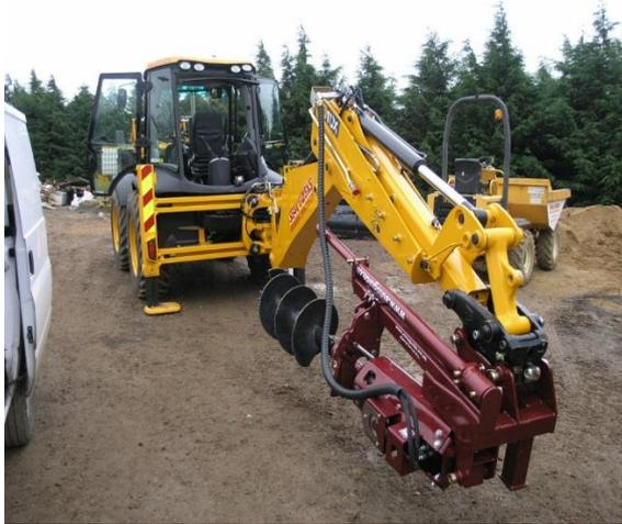
With the advancement of technical equipment, there is increasing use of excavator mounted augers. These can be used application where it is required to bore under shorter crossings such as under other utilities. This would involve open cut trenching up to the required bore are on each side and then lowering in the auger into the open trench to undertake the bore.
