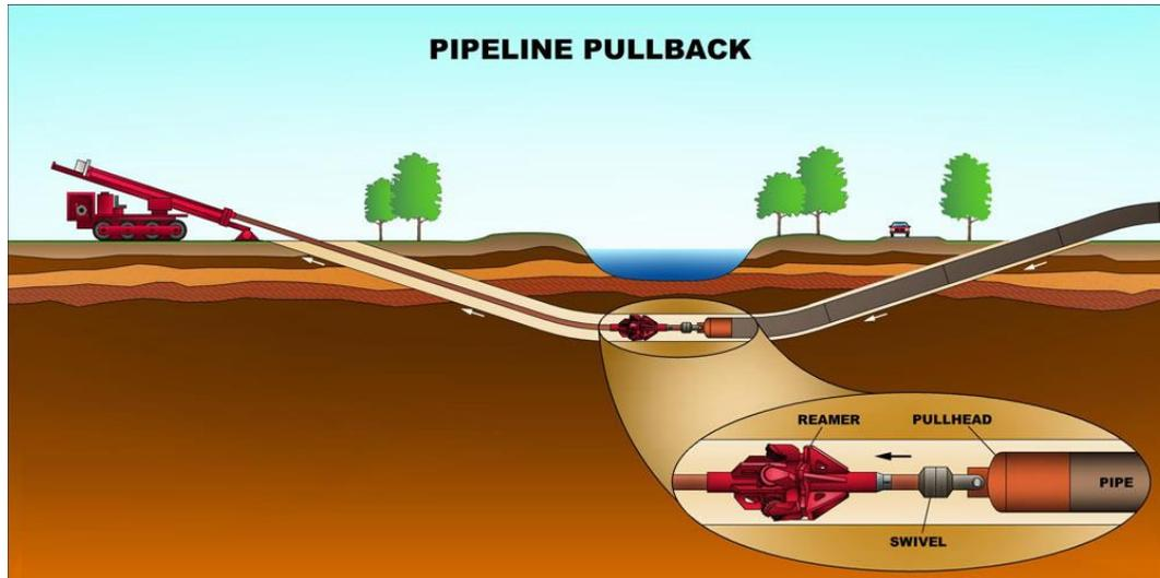
HDD is used for the installation of pipes and utility lines and is characterised by its use of a surface-mounted drill rig that launches and places a drill string at a shallow angle to the surface and has tracking and steering capabilities.
